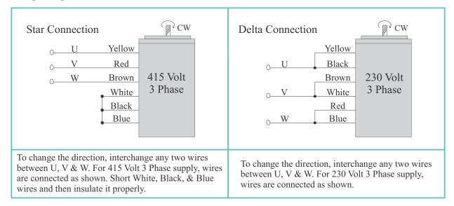
Change the direction of motor only after it stops rotating. If the attempt is made during rotation, motor may not change the direction or change the direction after some time.
